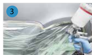
Clear Coat Application
