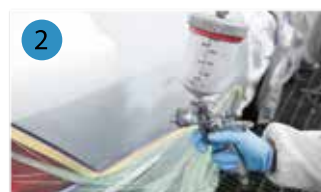
Base Coat Application
